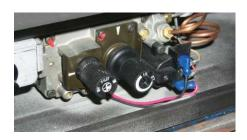
**11)** Remove the 10 Phillips head screws securing the valve access plate in place and then lift the entire assembly out.
